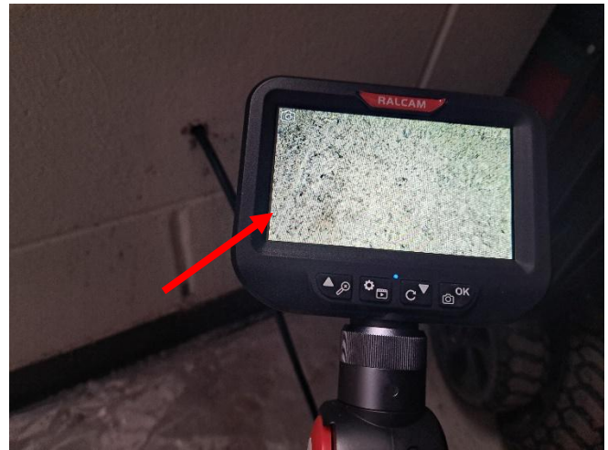
Photo 10: View of the concrete block wall during the vermiculite investigation and drilling activities (see arrow) within the library.
