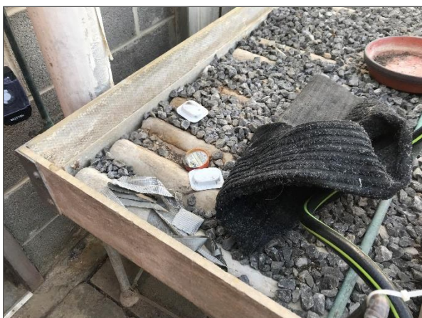
Presumed asbestos-containing Transite board present as gardening table.
