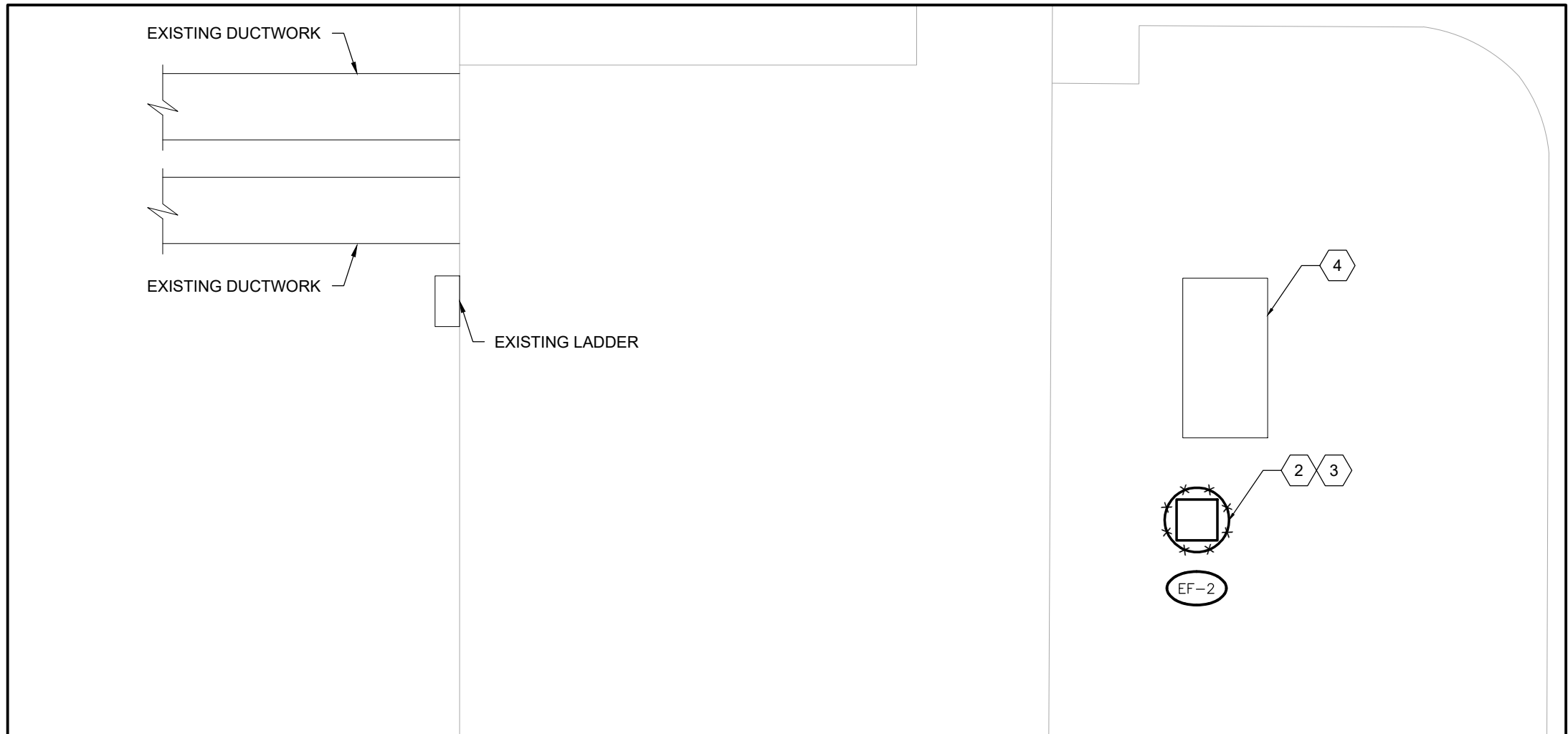
4 HVAC DEMOLITION PLAN - EXHAUST FAN - ROOF Scale: 3/16" = 1'-0"
