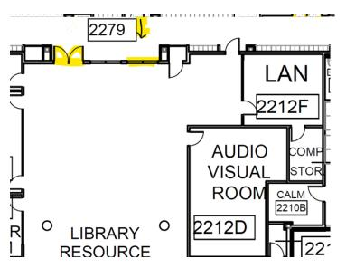
**Picture #1 Existing Window** - Remove and dispose the existing window and terrazzo tile base below the window, remove the concrete curb as required. Patch the floor with terrazzo and LVT flooring. Install a transition strip/threshold between the terrazzo and LVT. The finished work shall look like Picture #2 & Picture #3
