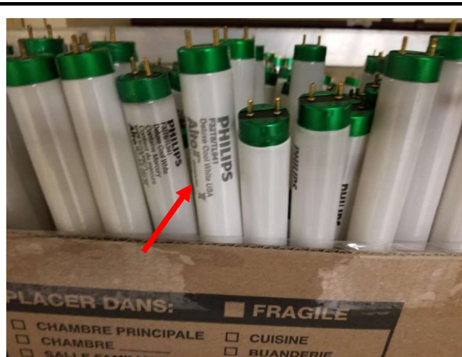
Photo 6: View of the mercury containing fluorescent light tubes (see arrow) observed to be in good condition throughout the Subject Building.
