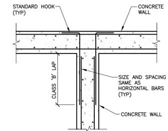
**TYPICAL PLAN DETAIL REINFORCING AT WALL INTERSECTION**
