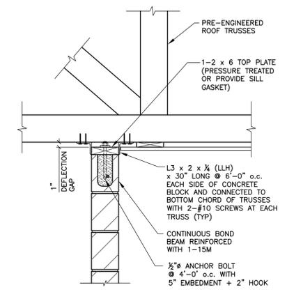
**LATERAL SUPPORT FOR NON-LOAD BEARING BLOCK WALLS PERPENDICULAR TO ROOF TRUSSES**
