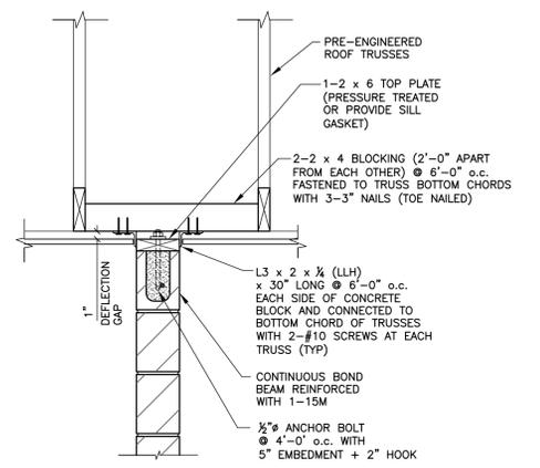
**LATERAL SUPPORT FOR NON-LOAD BEARING BLOCK WALLS PARALLEL TO ROOF TRUSSES**
