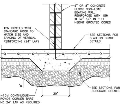
**SLAB ON GRADE UNDER NON-LOAD BEARING CONCRETE BLOCK WALL PARTITION**
