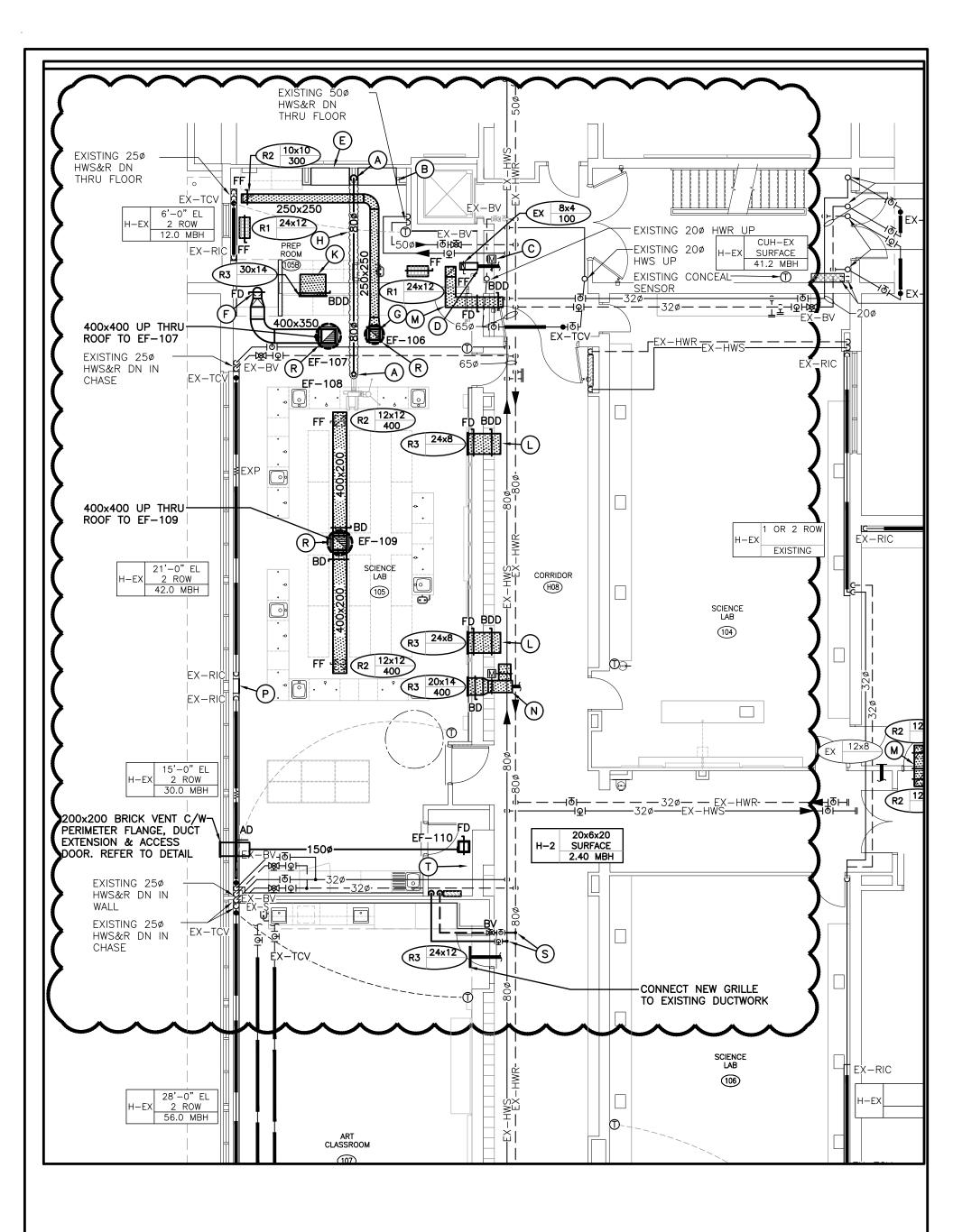
PART PLAN 'B' — HYDRONIC & VENTILATION RENOVATION SCALE: 1:100
